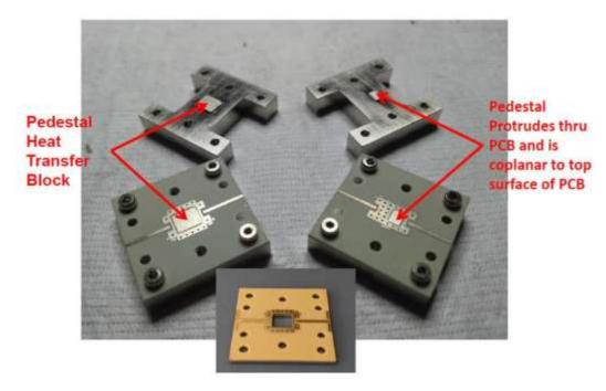
In cases where this is not possible, the foot print below may be used but the user's must account for proper power handling derating based on the maximum base plate temperature as outlined in the Absolute Maximum Rated table.
