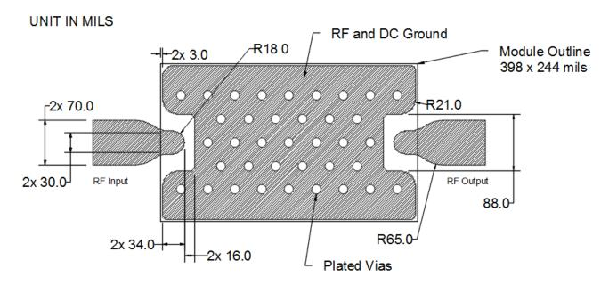
Low Signal PCB Layout Recommendation. Microstrip transmission line is based on Rogers 4003C, 32 mils, 1 oz copper. Minimum RF and DC ground illustrated. Plated vias are only sufficient for low signal evaluation. DXF available upon request.
