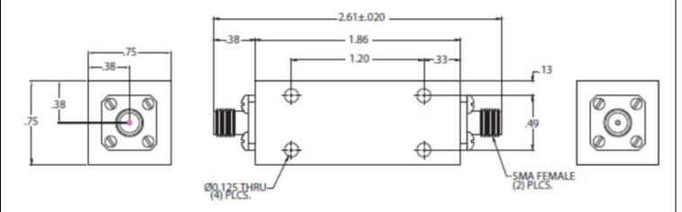
The RFLM-301511QA-392C SMA Connectorized package included input and output DC Blocking capacitors.
